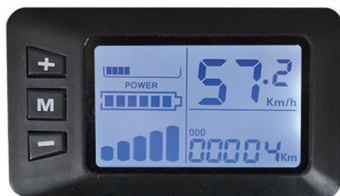
Model: G51 Size: 82.4mmx48.1mmx12.4mm Function: PAS Level; Speed; Trip/ODO; Headlight; Walk; Mile/KM; Error Alarm Communication: UART Holder: 22.2mm
